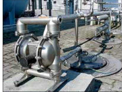
1 1/2" diaphragm pump installed in a chemical process to transfer chloride methylene
