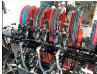
UL approved fuel pump 1" size, used assembled on skid dedicated in the aviation to fill and unload kerosene
