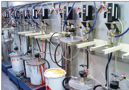
2-ball piston pumps 4:1 ratio, used in a painting process manufacturing
